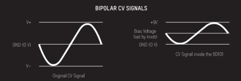
The incoming bipolar CV signal is shifted around the voltage that you select with the corresponding knob. Example: if you insert a -5V to a +5V sine wave into the CYCLE CV jack you will get the following results while turning the CYCLE knob:
