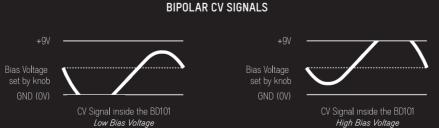
A similar thing happens to unipolar CV signals: their point of origin (0V) is shifted by the amount set with the corresponding knob. In other words: you add the voltage of your knob to the voltage of your incoming unipolar CV signal.
