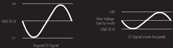
So, what happens? The incoming CV signal is shifted around the voltage that you select with the corresponding knob. Example: if you insert a -5V to +5V sine wave into the LFO SYMMETRY CV jack you will get the following results while turning the SYMMETRY knob:
