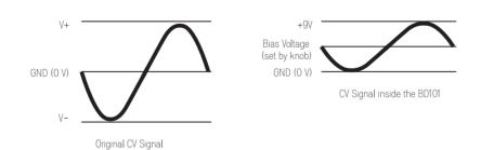
The incoming bipolar CV signal is shifted around the voltage that you select with the corresponding knob. Example: if you insert a -5V to a +5V sine wave into the CYCLE CV jack you will get the following results while turning the CYCLE knob:
