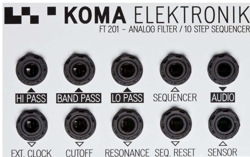
The patch bay consists of ten 1/4" mono jack sockets which you can use for receiving and sending various audio or control voltage signals. Blank arrows mark CV inputs/outputs, black arrows mark audio inputs/outputs. If the arrow is pointing towards the jack socket it shows you that this is an output, if the arrow is pointing away from the jack socket it is an input.
