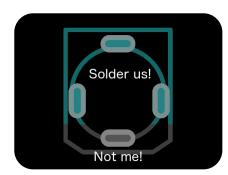
Next, we continue putting in the three types of toggle switches using the front panel to have them stand straight. Make sure the 'keyway' on the switches is always pointing left and you don't mix up the SP3T and DPDT switches (they can fit the same footprint). We can also already place in the LEDs so we don't have to take the front panel out once the toggle-switches are done. The LEDs should be placed in so that the long leg (anode, +) is facing left.
