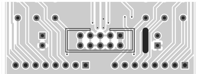
A close up of the Power Connector on the back side of the module.
