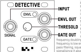
DETECTIVE is a simple Envelope Follower can he used to follow the overall shape of an input waveform and translate the changes in its amplitude to a DC voltage. You can use as a CV signal, or
