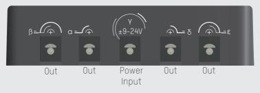
The back side contains the POWER INPUT in the center as well as the four DC OUTPUTS.
