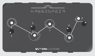
On the top you'll find the four Intensity controls - one for each channel - as well as four Channel LEDs and the Status LED.
